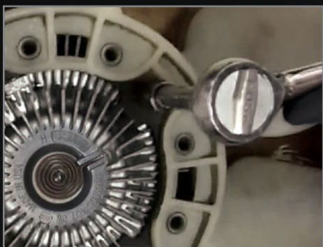
IMPROPER INSTALLATION: OVER TORQUE
